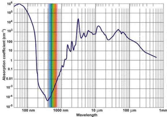
Fig 1. Light absorbtion vs wavelength curve
